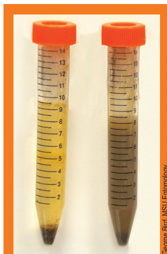
Figure 1. Field soil with excellent aggregate stability (left) and poor aggregate stability (right).
